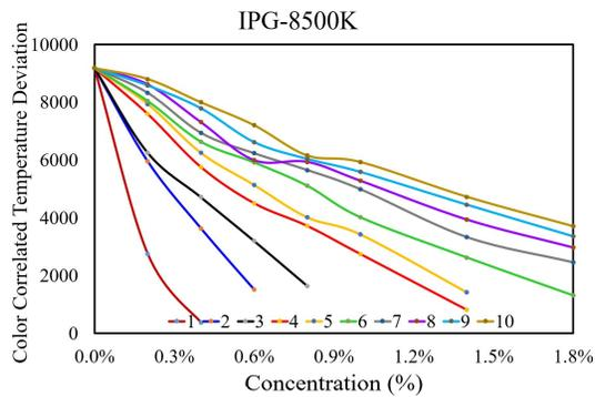
**Fig. 4:** The CCT deviation ( $\Delta CCT$ ) of MCW-LEDs at average CCT 8500 K with different LaTb particle sizes and concentrations.
